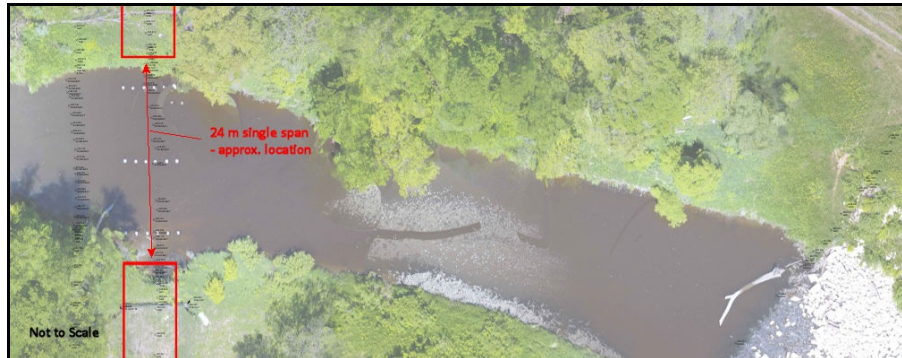
Figure 4. Proposed McEachern Bridge concept used for hydraulic studies (base sketch: adapted from Samson Engineering, 2024).
